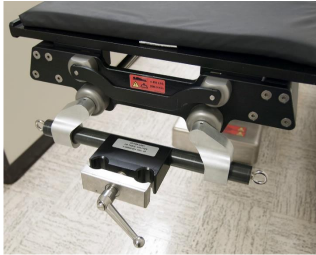
Figure 280: OR table adapter attached to mount
