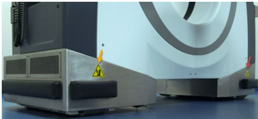
Figure 4: Identifying the scanner's safety label(s) – foot-crush-hazard label(s)
