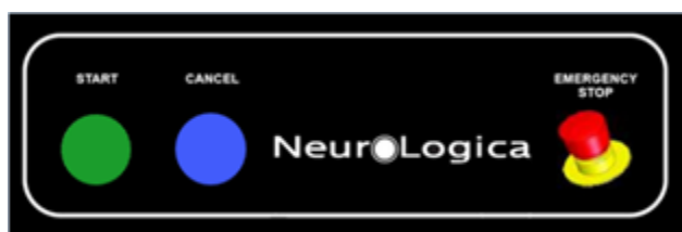
Figure 37: E-STOP button on the scanner control panel on both the left and right sides of the scanner
