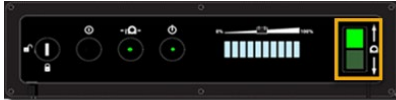
Figure 26: Rocker-Switch-Lift UP (top) and DOWN (bottom) button
