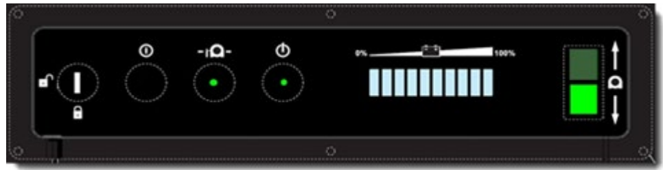
Figure 15: Operator control panel buttons and indicators
