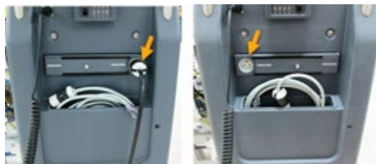
Figure 22: AC cord and storage on scanner (120V left plug in or 240V right plug out)
