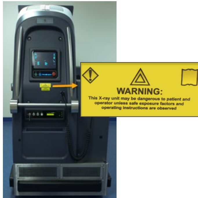
Figure 6: Dangerous-to-patient/operator safety-warning label location (left) and label (close-up, right)
