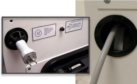
Figure 414: SDS retractable power cord —retracted (left) and not retracted (right)
