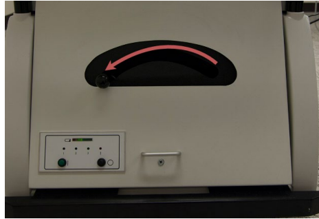
Figure 418: Locking lever in unlocked position
